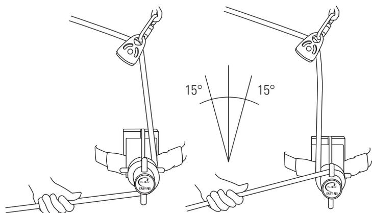
The **EASY RIG** should never be side-loaded. If it is necessary to use the **EASY RIG** on an adjacent tree (e.g. speedline setup) the rigging rope can be run through a pulley above the **EASY RIG** to prevent side-loading of the unit.
